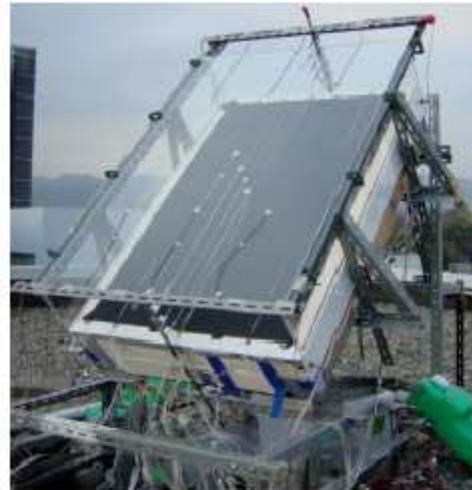
Fig.1: A photograph of the prototype solar chimney with built-in PCM modules for natural ventilation
